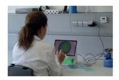
Regular colony counts are part of the day-to-day tasks of many laboratories in order to rule out the contamination of products with bacteria, viruses, yeasts, or molds during production. To do this, Petri dishes containing the relevant samples are evaluated in order to determine the number of colonies formed. While the classic manual counting method means that every single colony has to be marked individually, automatic devices can analyze numerous Petri dishes of the same type very quickly ...
