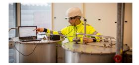
A new radio wave-based analysis technology, developed by the Finnish high-tech company Collo, makes it possible to continuously monitor the state of any liquid in industrial processes, be it thick slurries, resins, adhesives, coatings, emulsion, beer, water or any other fluid. Collo's technology is based on an electromagnetic resonator that emits a continuous radio frequency field into the liquid. The signal reacts to ...
