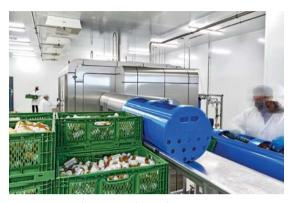
vessel. The vessel is filled with potable water and the pressure is increased to 6000 bar. This pressure is transferred from the water through the bottle into the product. With a dwell time of 180 seconds, such high pressure damages the cell membranes of bacteria and pathogens, inactivating the germs and resulting in a longer shelf life of the product. Parameters such as ...
